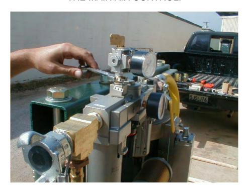
TIGHTEN REGULATOR IN PLACE WITH 11/16" WRENCH. STOP WHEN SNUG AND THE GAUGE FACES FORWARD.
