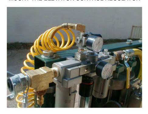
THREAD THE REGULATOR FITTING INTO THE OUTLET FITTING OF THE MAIN AIR CONTROL.
