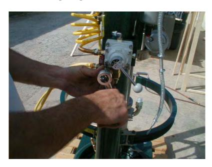
CONNECT THE AIR LINE TUBING. MATCH THE IDENTIFYING TAG OR TAPE STRIP TO THE FITTING, INSERT THE TUBE INTO THE FITTING AND PUSH UNTIL IT SEATS. IF YOU HAVE TO REMOVE THE TUBING, PUSH IN ON THE SMALL RING AT THE FITTING INLET WHILE PULLING OUT ON THE TUBING WITH THE OTHER HAND.
