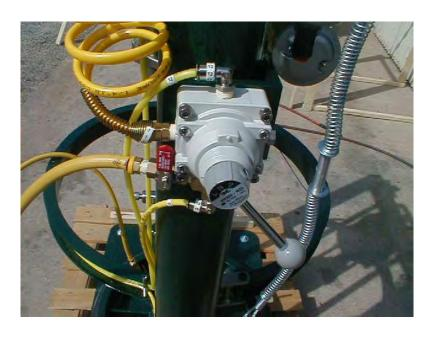
MOUNT THE VALVE WITH THE FOUR ALLEN HEAD CAP SCREWS PROVIDED. THE LOCK WASHERS BELONG UNDER THE HEAD OF THE SCREW AND ON TOP OF THE VALVE.
