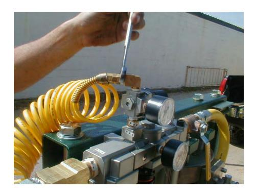
CONNECT THE COILED HOSE FROM THE ELEVATOR CONTROL VALVE TO THE REGULATOR. THE FITTING SWIVELS. USE A 9/16" WRENCH ON THE HEX CLOSEST TO THE THREADS.
