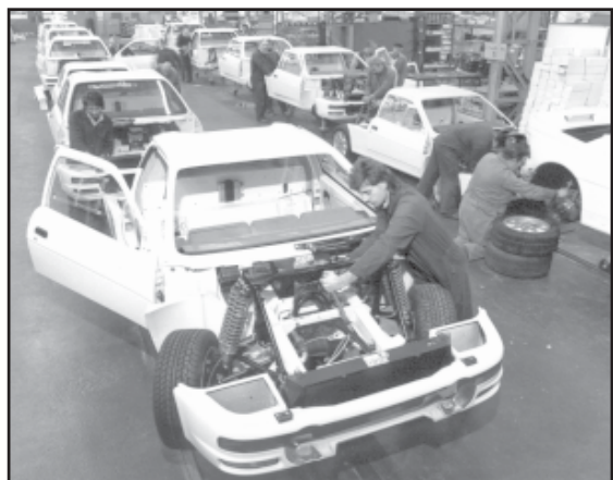
1986 Production of the (then new) Ford RS200 Group B rally car under way at the Reliant Motor Factory in Shenstone, Staffs -England.
