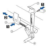
$\bigcirc$   $\rightarrow$  13 Nm / 10 Nm for carbon frame
