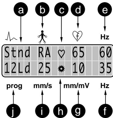
Figure 5-1. 12 Lead mode display
