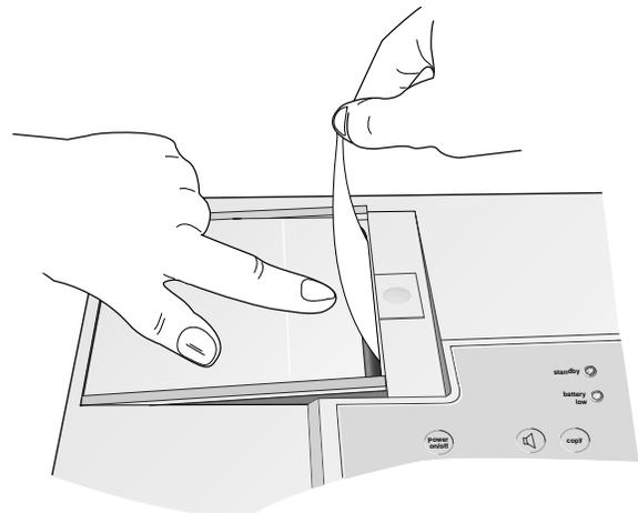
Figure 10-3. Closing the paper compartment
