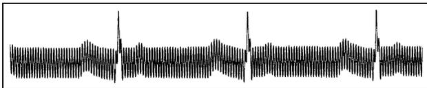
Figure 13-1. Regular AC interference
