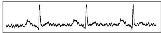
Figure 13-2. Irregular interference signals
