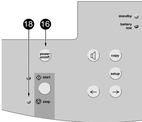
Figure 3-4. Operating controls and indicators
