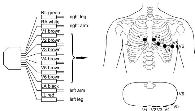
Figure 4-4. Connecting the patient cable (10-lead cable, standard leads)
