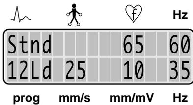
Figure 3-5. Display after successful MAC<sup>®</sup> 500 self-test
