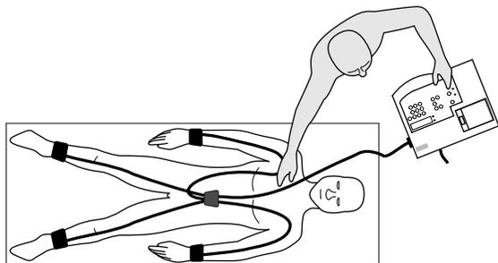
Figure 3-2. Arranging the MAC<sup>®</sup> 500 and examination couch
