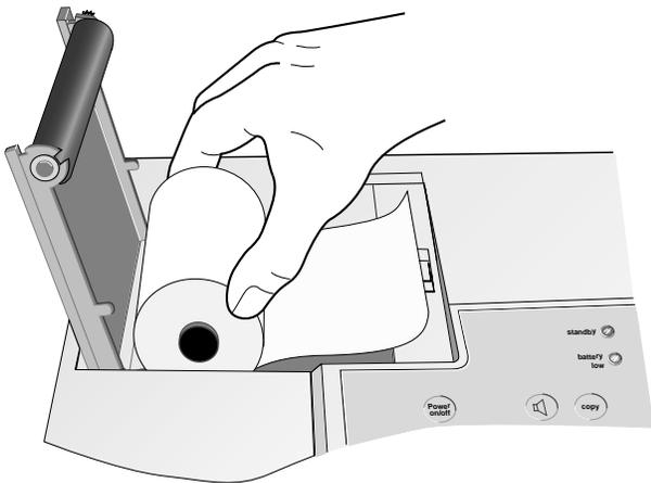
Figure 10-2. Inserting the new pad
