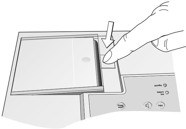
Figure 10-1. Opening the paper compartment
