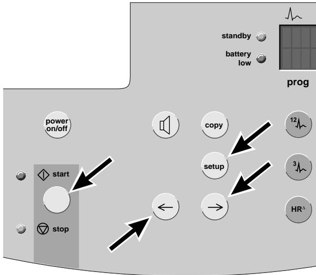
Figure 11-3. Recorder setup keys
