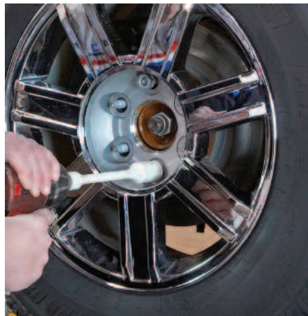
Torque the wheels to specification using a calibrated torque wrench or torque stick.
