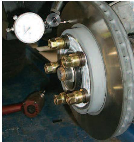
Measure LRO using a dial indicator.
