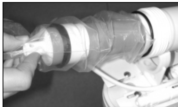
Figure 8 - Installing membrane without touching
