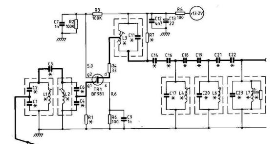
The modification involves removing one of the coupled tuned circuits on the input and re-arranging the connection point of g1 on TR1 (BF981). This reduces the loss from the antenna to TR1 by 1 to 1.5db. The modification is as follows:
