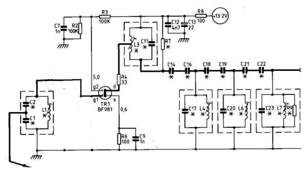
If all connections have been made correctly (double check) it is time to test. Connect power to the MX294 and switch on. Then connect a signal source and check the receiver is working OK, and then re-adjust L1 for best S/N on a weak signal. Though I did have an MX294 at one time with the BQF51 front end I did not get around to modifying it though I did write up the steps in my notebook. I will make this a subject of a future article in the club newsletter.
