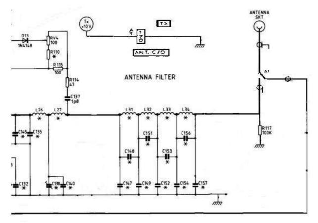
As can be seen from the diagram above all the diode switching components have been removed. On transmit Relay A is energised and contact A1 changes over the antenna socket connection from the TX to RX.
