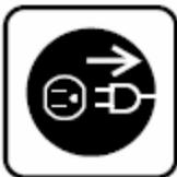
Always turn off and unplug the machine before moving, servicing, cleaning or any other conduct other than normal operation.
