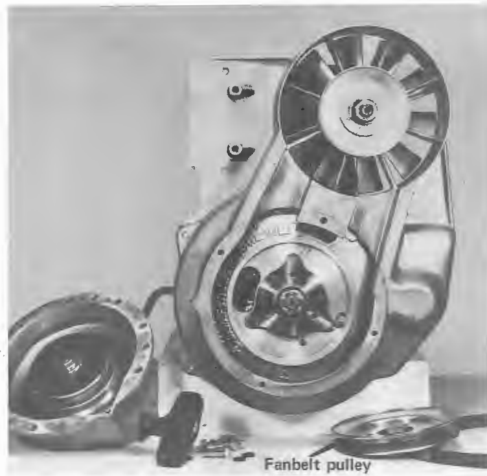
Fig. 3-4 Starter cup and fan belt pulley removed.
