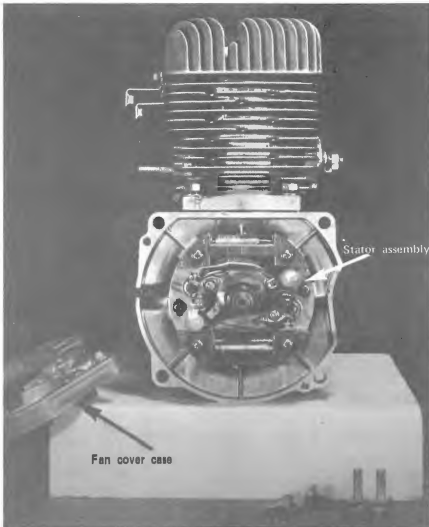
Fig. 3-7 Fan cover case removed
