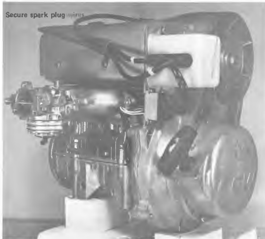
Fig. 5-12 Recoil Starter Installed
