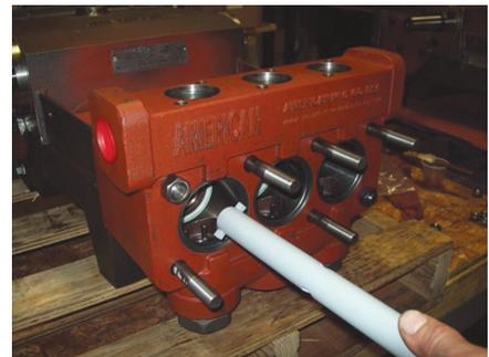
7. Pull the piston assembly free of the pump using a combination pulling and twisting motion.
