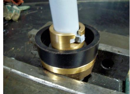
9. Inspect all parts for damage or unusual wear. Ensure that the interior surface of the cylinder (39) is smooth and free of cracks or grooves. New piston cups (40) will fail prematurely if installed in liners with damaged bores. American Mfg Company strongly recommends that all three piston cups be replaced, not just those that show signs of leakage, whenever this type of service is performed. This will maximize operational time between service intervals.
