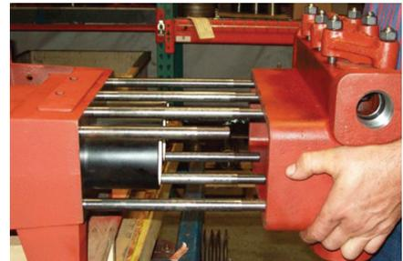
4. Rock the fluid cylinder (fluid chamber) to loosen from the cylinders (liners) (39), and then pull free of the fluid end studs. If the pistons have already been removed, take care to ensure that the cylinders (liners) do not fall off of the front of the power end and become damaged.
