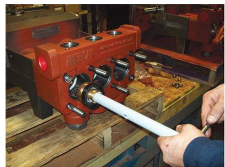
8. Place the flats on the bottom of the piston holder (41) in a vice or clamp securely. Using the American Mfg Company piston tool (PPFMC A5049), unscrew the piston retainer nut (43) and remove. The piston cup (40) and piston retainer (44) may now be removed.
