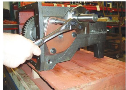
9. To remove the crankshaft (2) on AL1122 models work the crankshaft (2) to the left when viewing from the rear opening of the power frame. The throws or journals may have to be rotated as the crank is removed to clear the connecting rods (4). Slip the crankshaft end on the right out the back of the power frame and remove. The crankshaft (2) should be handled carefully to prevent the critical bearing surfaces from being scratched or damaged.
