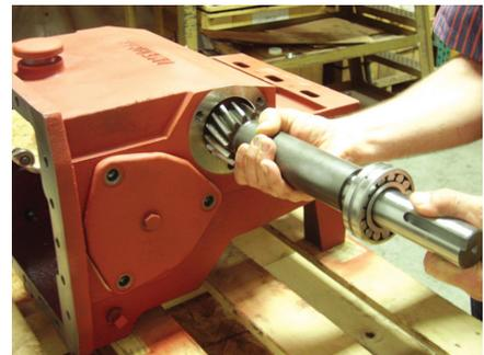
7. The pinion shaft (3) with bearings may then be removed from the drive side by using a brass rod (or other soft material) and mallet to drive the shaft out.
