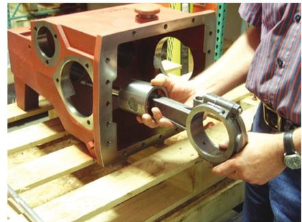
12. Remove the set screw (21) and slide the wrist pin (6) out of the crosshead (7) if crosshead or connecting rod (4) requires service. Keep components matched together.
