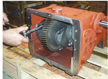
5. Slide the two rod bearing halves (5) from each connecting rod (4). Note that these parts sometimes adhere to the pins (journals) on the crankshaft (2).
