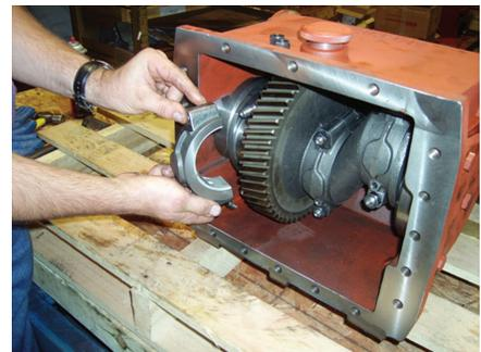
**NOTE:** Connecting rods and caps are matched sets and must always be reassembled with their original mate and in the same orientation. Note the numbered codes stamped on each half of the connecting rod assemblies and make certain they are installed as matched set and in the same orientation when re-assembling the pump.
