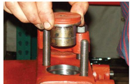
6. For ball valves, the balls are not retained in the valve seat. The ball can easily be removed from the valve assembly by lifting it out of the open cage portion of the valve seat with American Mfg Company tool PPAM A000239000.
