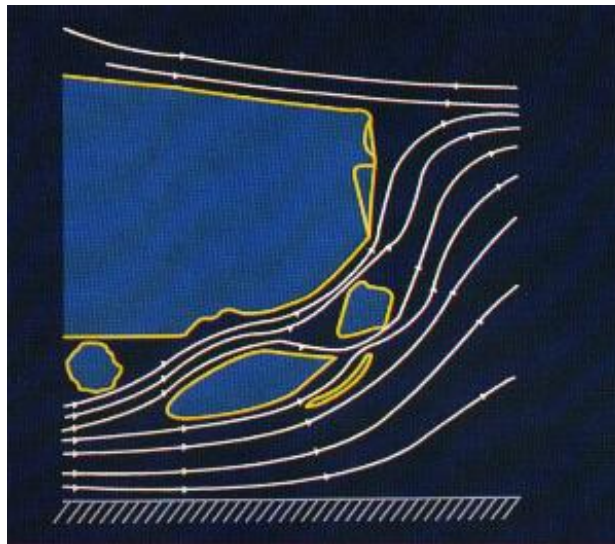
Air flow pattern around the Z1 rear exhaust box and body panels
