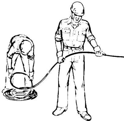
Figure 4-27. Incorrect Method of Unreeling Wire Rope
