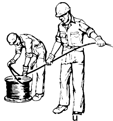
Figure 4-28. Incorrect Method of Uncoiling Wire Rope
