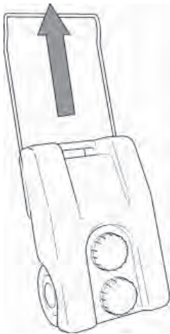
Fig. 5 Open handle and wheel to water supply. Remove blank cap and fill.
