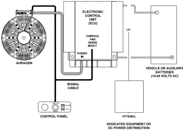
**Inverter Charger System (ICS):** Provides 120 or 240 VAC and 14 or 28 VDC power with or without engine running. An optional remote power strip with 120 or 240 VAC service is also offered.
