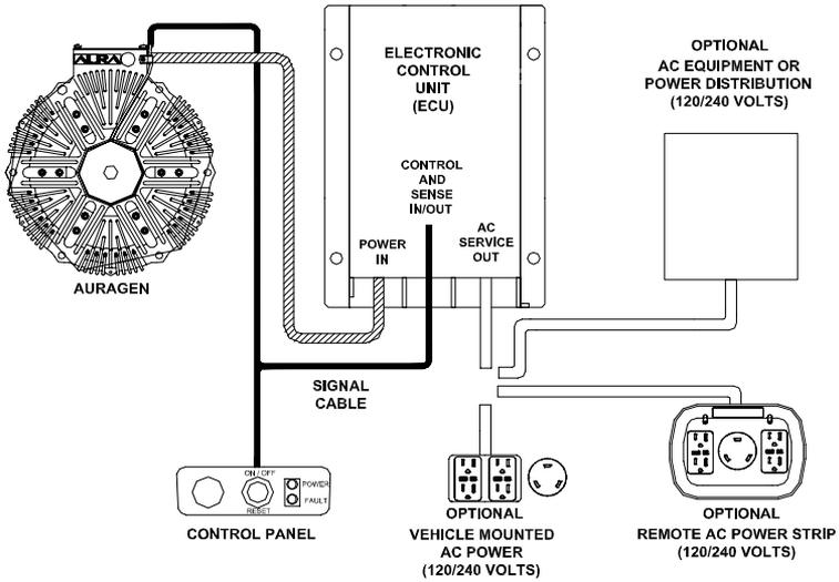
**AC/DC:** Provides 120 VAC power to GFI outlets and 14 or 28 VDC connected to the vehicle batteries. An optional remote power strip with 120 VAC service is also offered.
