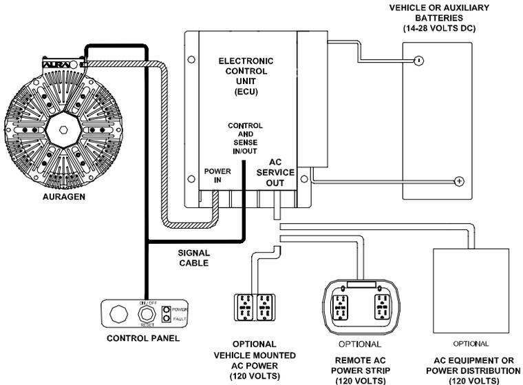
**All-DC:** Provides 14 or 28 VDC to auxiliary batteries. No AC service is available.
