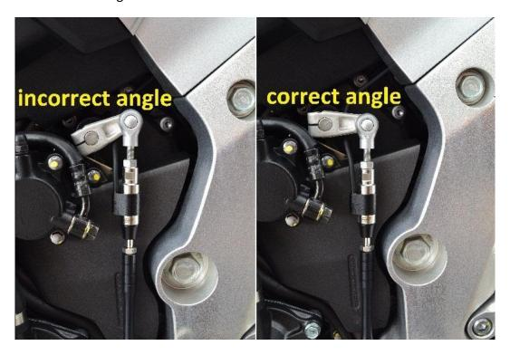
**NOTE**: The gearbox pivot arm must extend to 90° degrees with the rose joint in order to receive an equal force in both directions, if not set corectly, the gearbox may not react accordingly and miss gears when using the quickshifter!
