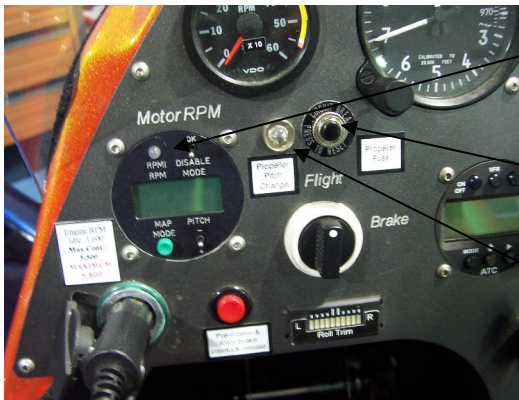
View of left side of panel if fitted with Woodcomp propeller and CSC-1 controller
