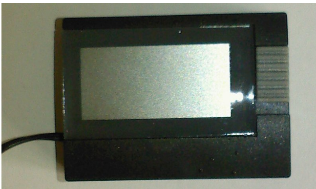
View of front, prior to panel fitment. Unit is bonded to panel. Switch should be down – this changes the unit between deg C and deg F
