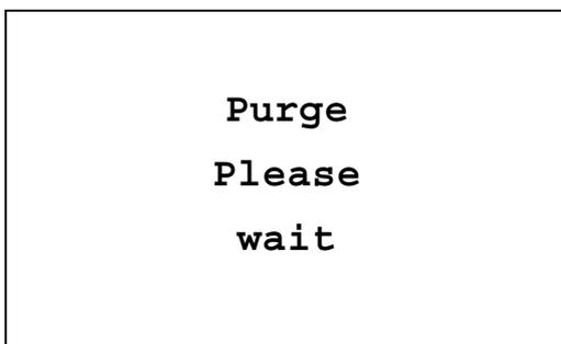
After successful purging ( HC < 20 ppm ), device switches off automatically.
