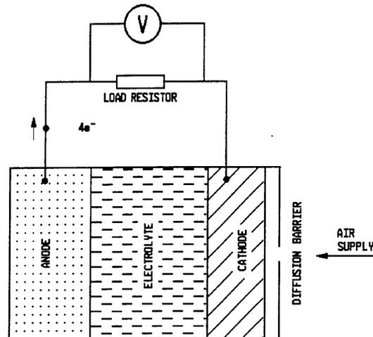
**Picture 2: Principle of the electrochemical sensors of the DELTA 1600 S-IV**
