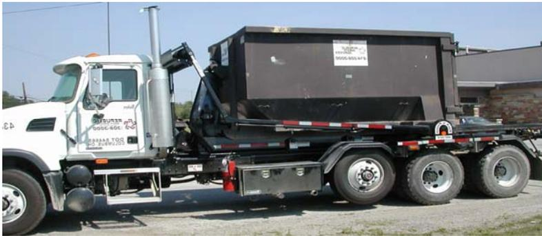
if so, move container to the rear of the frame by moving the carriage rearward,
