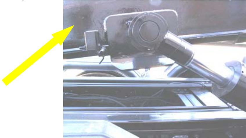
2. Raise the hoist and verify the service props hang straight down (vertical).
