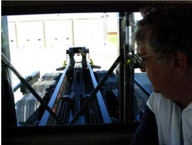
7. With the container long sills in contact with the hoist rollers, continue to lower the hoist and move the container further onto the hoist frame by moving the carriage forward.
