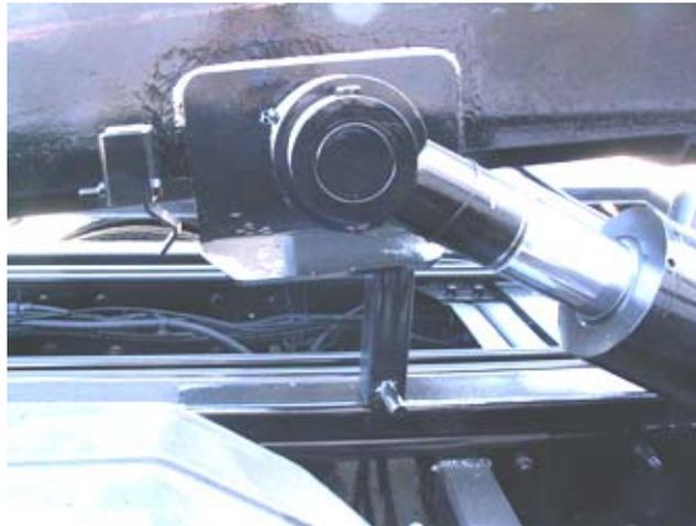
Lower the hoist and visually check to make sure that BOTH props are correctly inserted into the retaining fixture. If the service props do not fall into place inspect them to make sure they are not damaged. If damaged, DO NOT perform any other maintenance until they are repaired and in good working order. If the service props are not damaged then manually align them with the retaining fixture.
