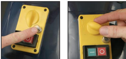
If the cutting blades are jammed turn the rotation direction switch to position
