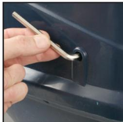
2. If you are shredding heavy materials (such as harder or large materials) they may need to be put through the shredder twice, to crush the material before cutting it completely. To loosen the adjusting screw, turn the allen key anti-clockwise half a turn, in the CRUSH direction.
