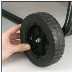
4. Position the remaining washers and the locking nuts (16) on each end of the axle and tighten both the wheel nuts using a suitable spanner.
