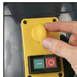
Push in the overload protection button (3) to re-set, mains power can now be switched on.
