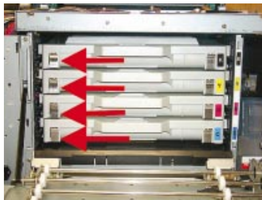
Figure 3 - Bend out toner cartridge tabs (denoted by arrows).
