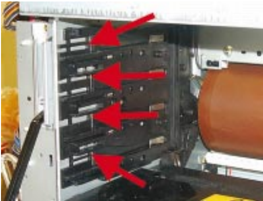
Figure 2 - Arrows denote toner key sensor tabs.
