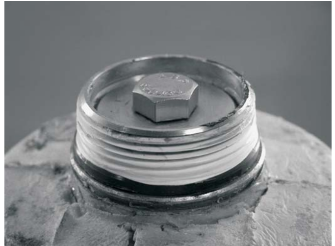
Top of Bearing Thrust Washer
