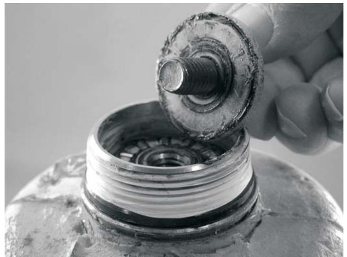
Thrust Washer and Bearing
