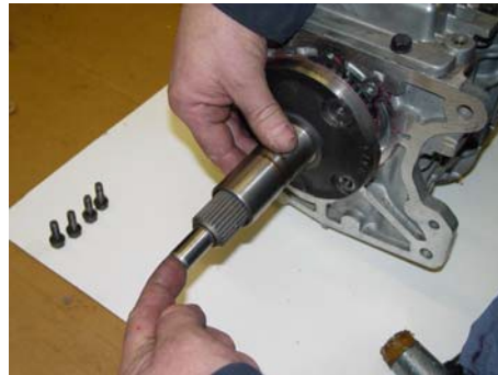
FIG. B REMOVE OLD RETAINER
