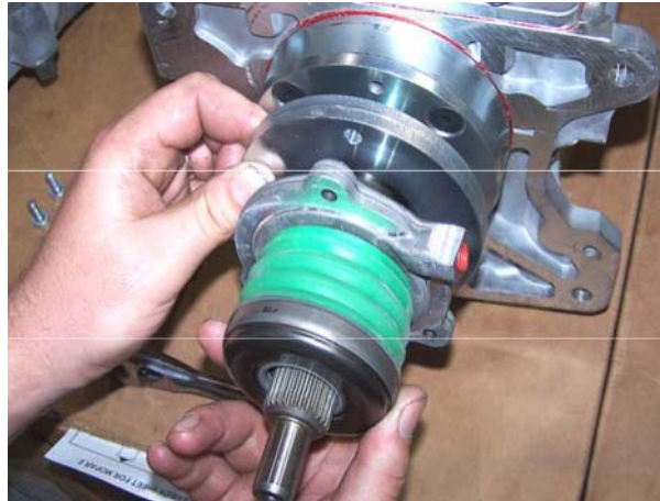
INSTALL SPACERS IF NEEDED
