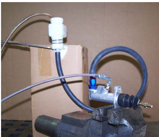
MASTER CYLINDER AND RESERVOIR MOUNTED FOR BENCH BLEEDING
