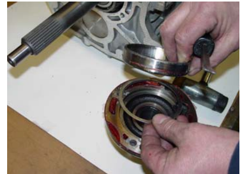
FIG. C (TKO ONLY) REMOVE BRG. RACE AND SHIMS
