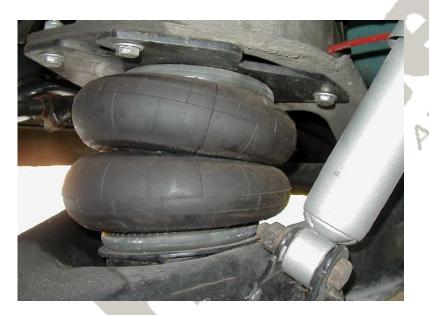
3. Hold the upper plate to the cross member as shown in the picture to the left and clamp to frame. Using the plate as a template drill 4 holes in the cross member.
