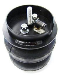
3. Apply thread sealant to a 90 degree air fitting and screw it into the top of the air spring.
