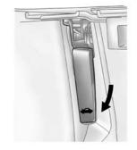
1. Pull the interior bonnet release handle located to the left of the steering column below the instrument panel.
