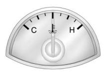
This gauge shows the engine coolant temperature.
