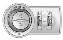
The exterior lamp control is located on the instrument panel on the outboard side of the steering wheel. Turn the control to the following positions:
