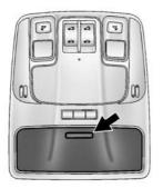
Push on the cover and release to open the compartment.
