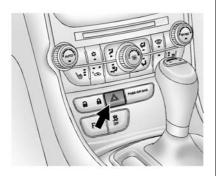
(Hazard Warning Flasher): Press this button located on the instrument panel above the audio system, to make the front and rear indicator lamps flash on and off. Press again to turn the flashers off.
