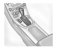
The automatic transmission has a shift lever located on the console between the seats.
