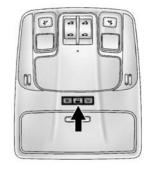
The interior lamps control located in the overhead console controls both the front and rear interior lamps.
