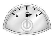
When the ignition is on, the fuel gauge shows how much fuel is left in the fuel tank. When the indicator nears empty, a message in the Driver Information Centre (DIC) displays. See *Fuel System Messages on page 4-38*. The vehicle still has a little fuel left, but the vehicle should be fuelled soon. An arrow on the fuel gauge indicates the side of the vehicle the fuel door is on.
