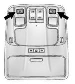
The reading lamps are located in the overhead console.
