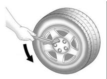
Turn the wheel wrench anticlockwise to loosen all of the wheel nuts, but do not remove them yet.
