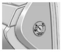
This switch should only be turned to the OFF position if the person in the front outboard passenger position falls under the conditions specified in this manual as follows:
