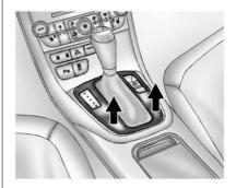
2. Release the gear lever trim from the centre console at the rear, then fold upward and rotate to the left.
