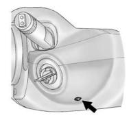
Vehicles with an automatic transmission are equipped with an electronic key lock release system. This system is to prevent ignition key removal unless the gear lever is in P (Park).
