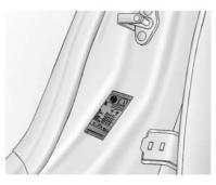
The recommended tyre pressure is shown on the label attached to the vehicle's centre pillar (B-pillar). See *Vehicle Load Limits on page 8-10* and *Tyre Pressure on page 11-6* for more information. The tyre pressure data refers to cold tyres.
