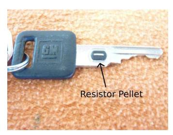
There are 15 different pellet used in these keys. They are idenitifed by the amount of resistance in the pellet.
