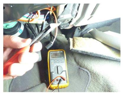
Cut the end of the lock cylinder harness off.
