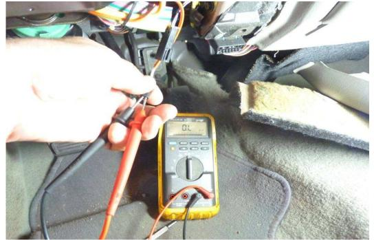
Unplug the connector and ohm the wire that goes to the ignition lock cylinder. With no key in the lock cylinder, It should read open or OL (out of Limits).
