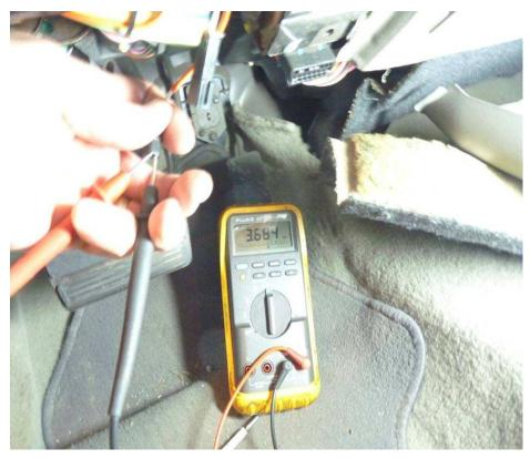
With the key in the lock cylinder, It should read out the same or very close to the same as you ohmed the key. Rotate the key and make sure the resistance stays the same and does not go open. You can see this ohms the exact same as the key. If it would give a different resistance or stayed open, that would mean the wire for the lock cylinder may be broken inside the steering column.
