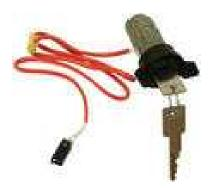
The Ignition lock sensor has 2 wires attached to it that runs down the steering column. These wires are known to break from the turning of the ignition switch. If one of these wires gets broken, the security light will come on and the car may not start.
