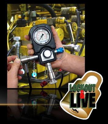
The only way to insure a hydraulic system is safe to work on, after the prime-mover has been locked out, is for a worker to have the ability to verify if there is stored energy, and remove the stored energy if necessary, at the point-of-work.
