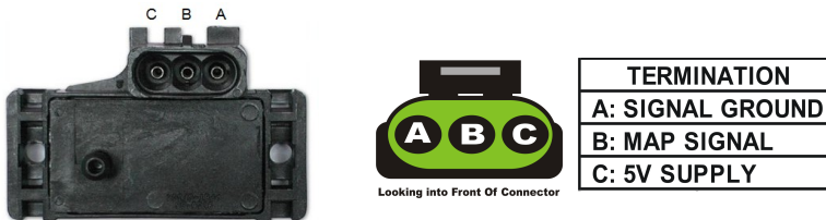
Figure 5 – Manifold Absolute Pressure Sensor and harness Termination
