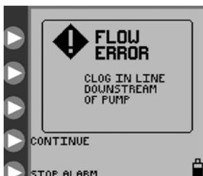
Figure 27. Flow Error screen.
