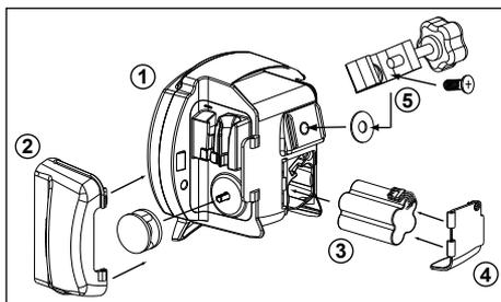
Figure 34. User Serviceable Parts.
