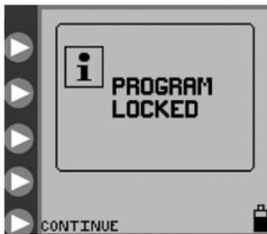
Figure 19. Program Locked screen, which indicates the pump is in LOCK SETTINGS mode.
