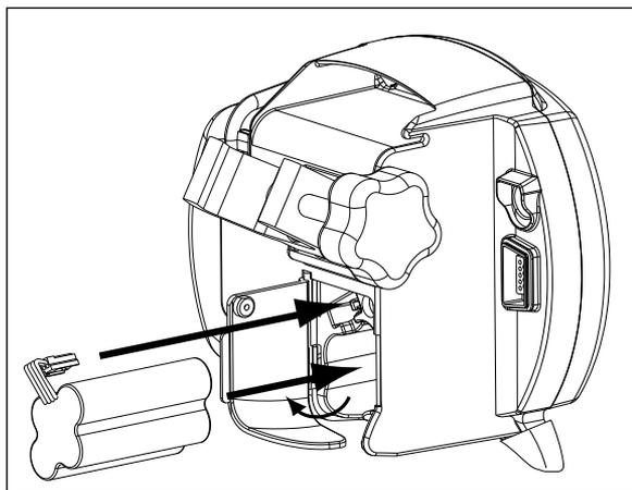
**Figure 21. Installation of Battery Pack.**
