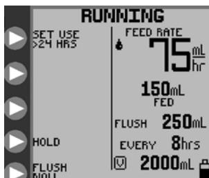
Figure 14. **RUNNING** mode screen for continuous feed mode.
