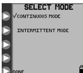
Figure 9B. **SELECT MODE** menu for continuous or intermittent mode selection.
