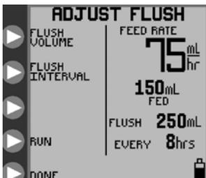
Figure 11A. *ADJUST FLUSH* menu, continuous mode.
