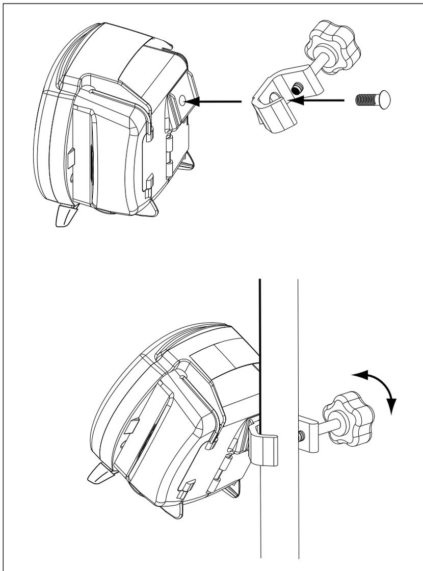
**Figure 3. Attaching and using the Pole Clamp.**
