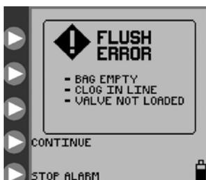
Figure 26. Flush Error screen.
