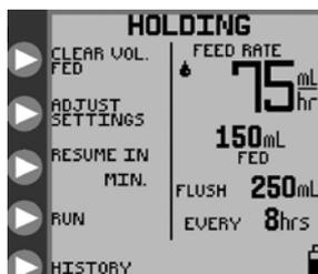
Figure 15A. **HOLDING** mode options, continuous feeding mode.
