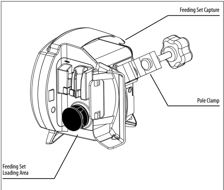
Figure 1B. KANGAROO ePump Pump Set loading area.
