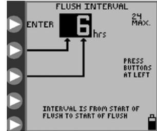
Figure 11C. Setting the Flush Time Interval.
