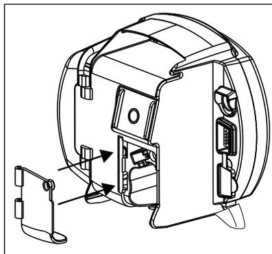
Figure 33. Battery Door Replacement.
