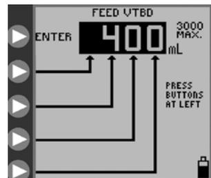
Figure 10C. Setting the Feed Volume to be Delivered.
