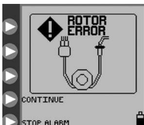
**Figure 24. Rotor Error screen.**
