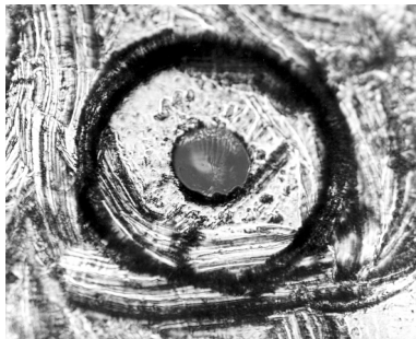
Figure 4-7. Damage from improper cleaning.
