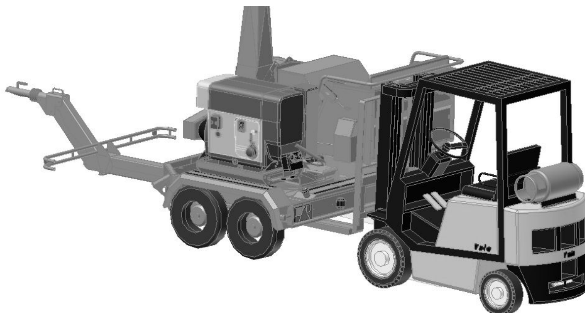
Figure 5 Lifting with a fork lift truck
