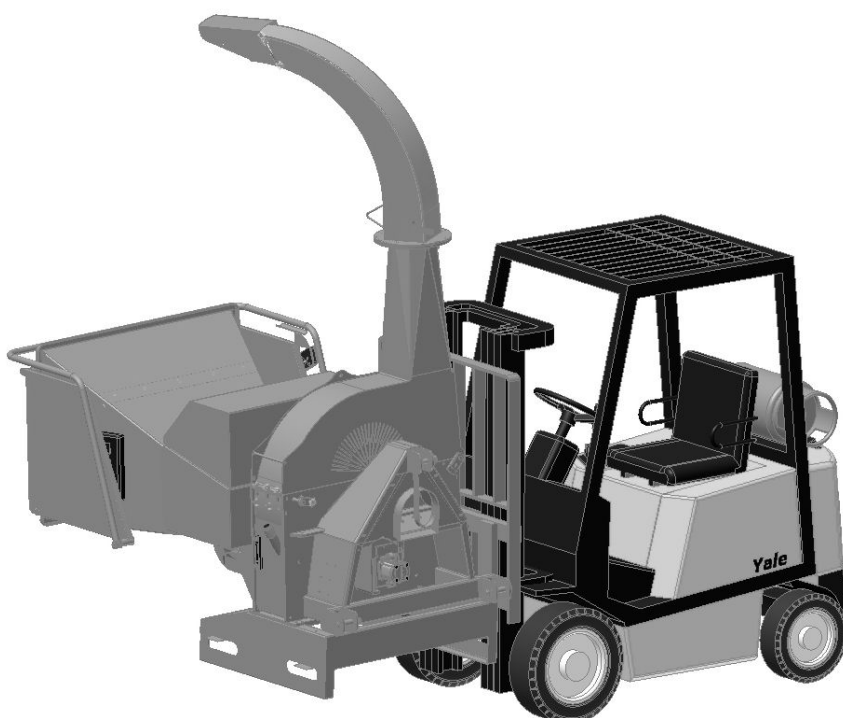
Figure 4 Lifting with a fork lift truck
