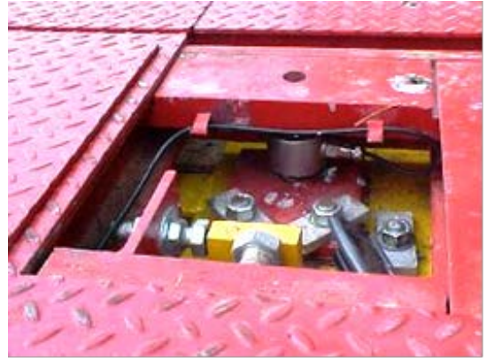
Load Cells are preinstalled and pre-wired, located under the plate
