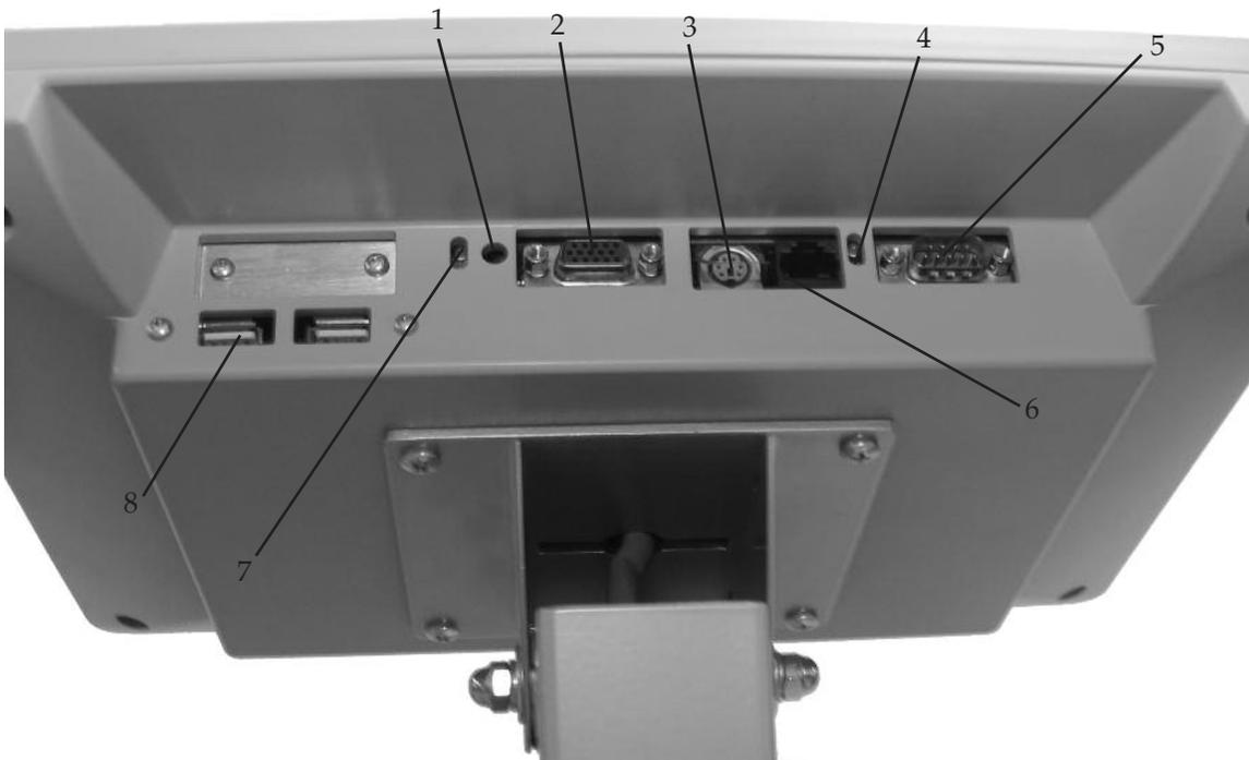
Figure 3.1. The printer power cable should be plugged into the AC receptacle on the rear base of the display support post. The printer USB cable should be plugged into the USB port on back of the display.
