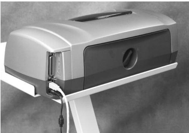
Figure 3.2. Connect the power cable and USB cable to the rear of the printer.
