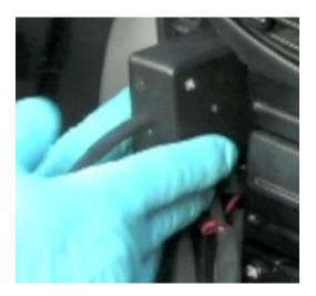
C. Connect your IMS Guardian™ Switch (already installed into the switch panel) to the wire harness.
