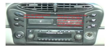
B. Remove switch panel from console. The panel simply pops out by prying against it with a flat head screwdriver. Care must be taken to avoid scratching the console.
