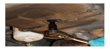
STEP TWO: Remove, Inspect and Clean The Sump Plate
