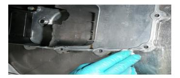
STEP 6: Reinstalling The Sump Plate
