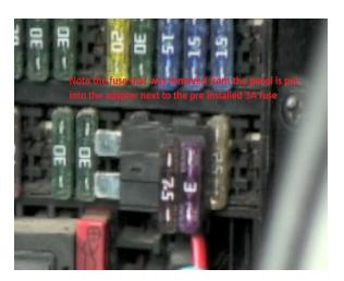
D. Install the fuse adapter in the fuse panel.
