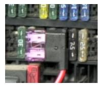
E. Route the main power lead (red wire) through the fuse panel cover.
