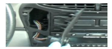
C. Remove one of the blank block out plates in the switch panel.
