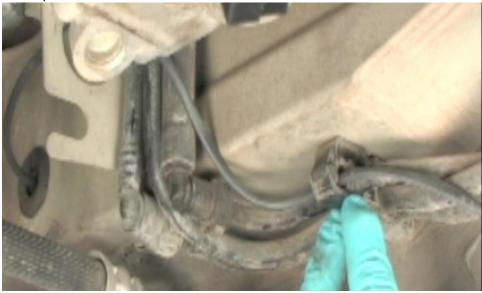
STEP 18: Connecting The Wire Harness To MCD
