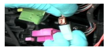
C. Connect the white connector coupler into the black connector coupler of the orange power lead wire.
