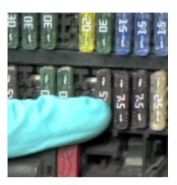
C. Using the fuse adapter on the IMS Guardian™ wire harness, reinstall the removed fuse into the adapter.
