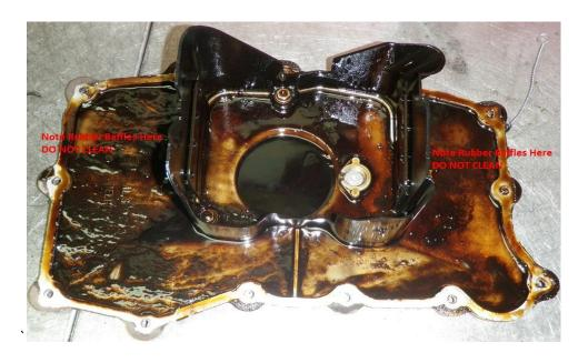
STEP 3: Inspection Of Oil Sump and Pickup Tube
