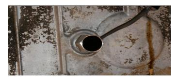
STEP 8: Remove / Change Your Oil Filter and Fill Engine With Oil
