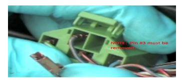
B. Connect the white connector coupler (included) to the spade terminal removed from the switch connector. (NOTE: Be sure beveled edge of the connector coupler faces the lock of the spade connector.)
