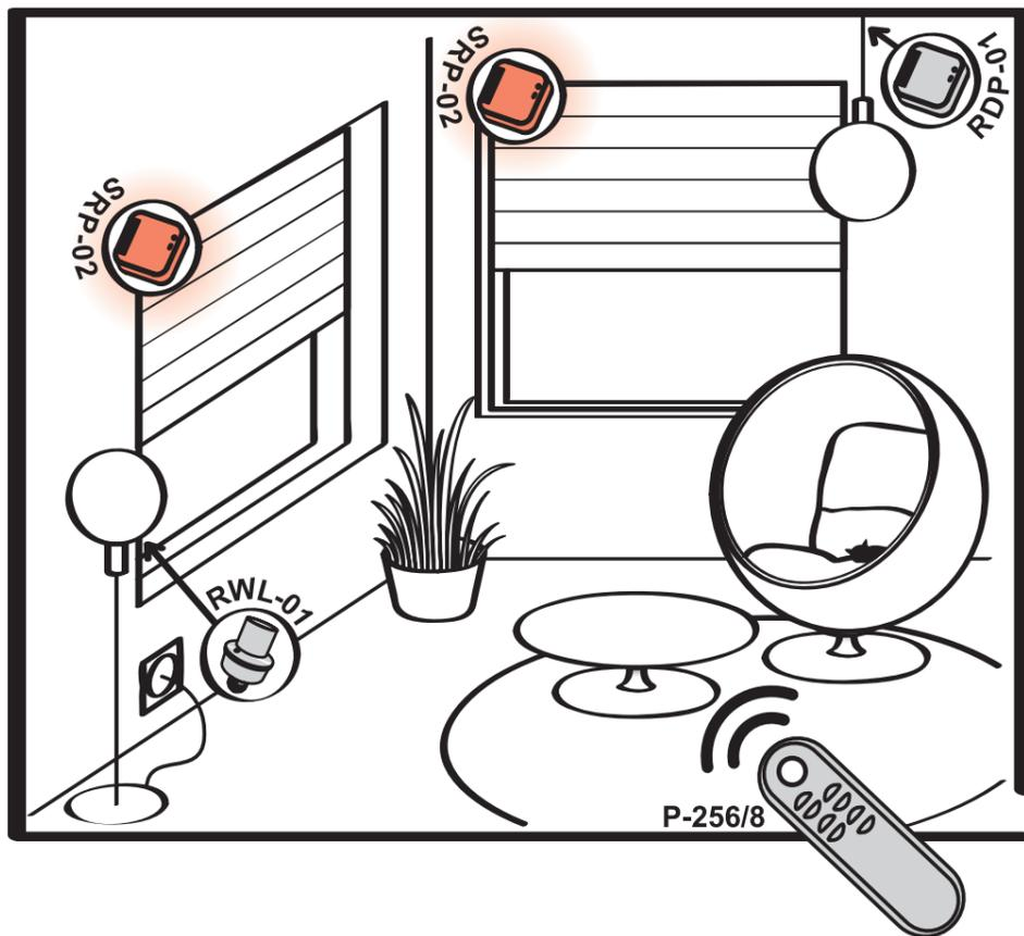
Roller blinds control system realised by means of SRP-02 roller blinds controllers. One controller can be used for one roller blind. Each of the controllers is operated by means of a wireless P-256/8 remote control. The remote control can also control operation of RDP-01 radio dimmer (switch on /switch off control and light sources brightening / dimming) and of RWL-01 radio lighting switch.
