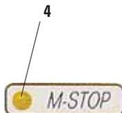
If the yellow LED in the **M-STOP** field (4) of the control panel is lit, the mechanical handwheel lock or the handwheel brake (Item 3 in Fig. 3) is activated.
