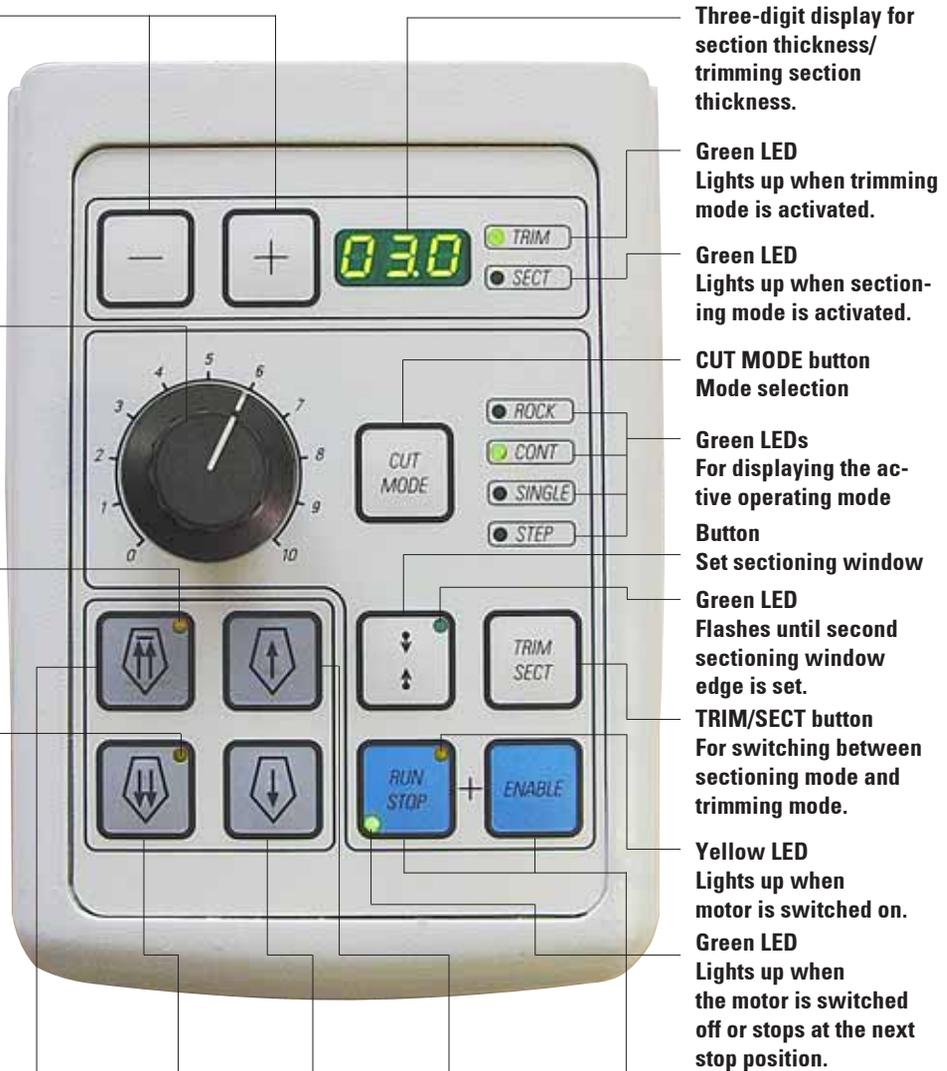
**Three-digit display** for section thickness/trimming section thickness.
