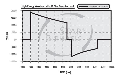
The Biphasic Truncated Exponential (BTE) waveform uses variable energy. The actual energy delivered will vary with the patient's impedance and the device will deliver a shock when impedance is between 25-180 Ohms. Energy will be delivered at three different levels referred to as ultra-low variable energy, low variable energy, and high variable energy as shown in the waveform tables below.
