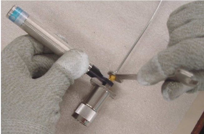
Fig. 3-6 Connect the coax assy A (item 04) to the N-SMA connector (item 09) using a torque wrench
