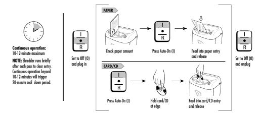
Breakthrough Safety Technology! Safe Sense™ stops shredding when hands are too close to the opening. © Override switch - is only needed when a jam occurs and Safe Sense™ light remains on. Warning - when switch is in override position the Safe Sense™ light flashes and the Safe Sense™ feature is rendered un-functional.
