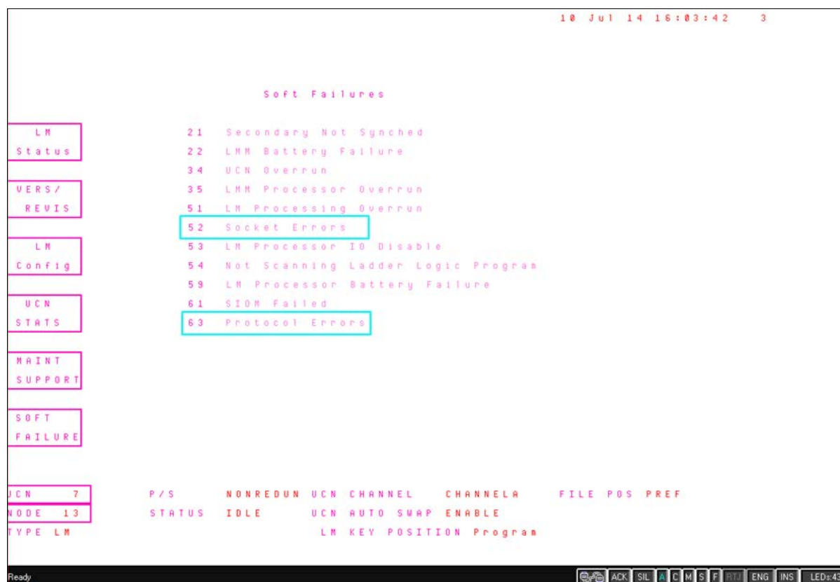
Figure 6-1: SOFT FAILURE Display for Enhanced Logic Manager
