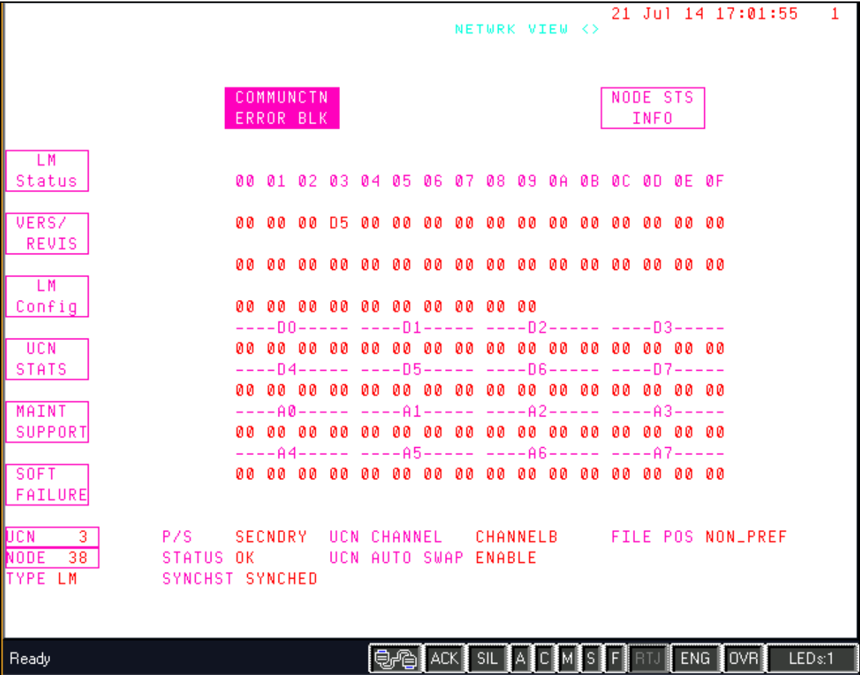
Figure 6-8: Enhanced Logic Manager Communications Error Block Display
