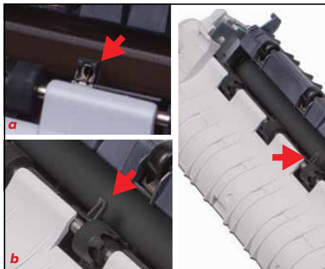
The 4250 fuser exit sensor flag, a, is unique.
