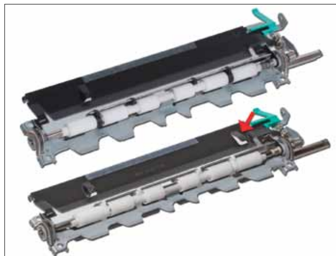
REGISTRATION ASSEMBLY. On top, RM1-0011-R, the original 4200/4300 registration asm. Below, RM1-1098, showing the clearance notch that makes it compatible with 4200 and 4250 printers alike.
