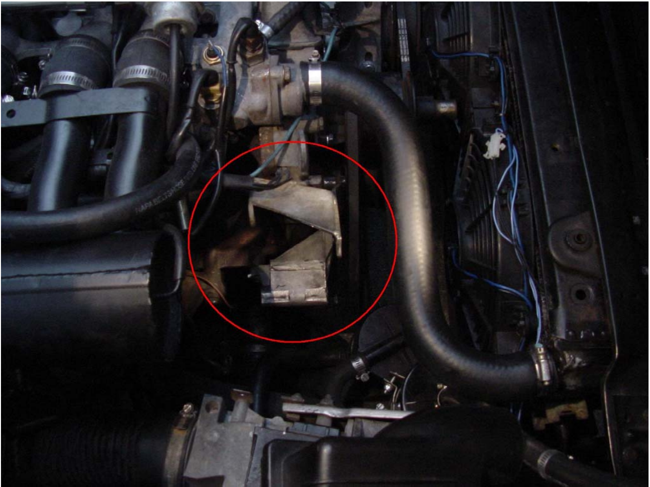
Picture 1: Old alternator removed from engine mounting brackets.
