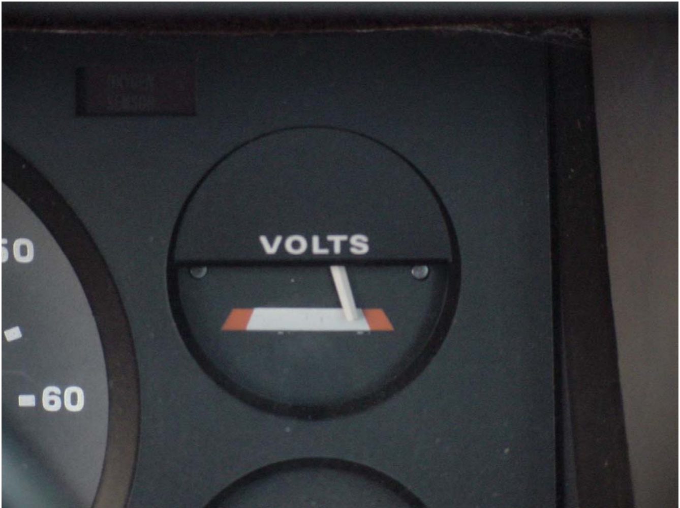
Picture 7: TR7's Voltage Meter, pointer location showing the Alternator is "charging" the battery.
