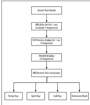
1. All LED's light up and it sends out Beep Sound when it enters into the Quick Test Mode. (Including 7-Segment)
