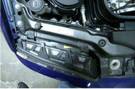
2. Start by opening the hood and locating the (4) mounting screws that hold in the headlight. Removing the headlight will make the installation process much easier.
