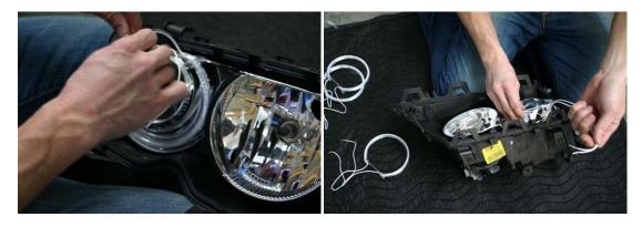
5. Clip the Angel Eye rings onto the reflector housing. If equipped with auto-level feature, make sure there is enough clearance for the projector to move up/down without coming in contact of the ring.
