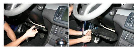
20. Remove the trim underneath the steering wheel to gain access to the LCM wiring.
