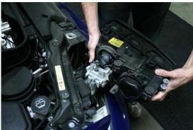
Remove the corner lens. This will either be a screw type (Phillips) or push in design. The screw type will simply unscrew off, the push in have a retaining clip that is pushed down to remove the lens. Remove lower headlight trim by unclipping the inner tab closest to the kidney grilles. Then release the outer clip of the lower trim by pressing on the outer tab using a pick tool. Once trim is detached, the headlight can be removed.
