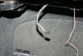
18. Unplug the connector going into the footwell lighting and tap into the red wire of the connector with a scotchlock or solder into place. Reconnect the connector to the footwell lamp and reinstall the glovebox back into place.
