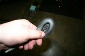
17. Remove the oval grommet and poke a small hole for the trigger wire to pass through the interior opening. Route the wire through the opening and replace the grommet back into place.
