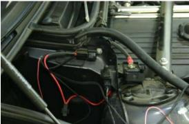
12. Connect the power wires and test the Angel Eyes before routing the cables. Connect the larger gauge red to the +12V positive and the black to chassis ground. The small red/white wires going to a +12V source temporarily for testing.
