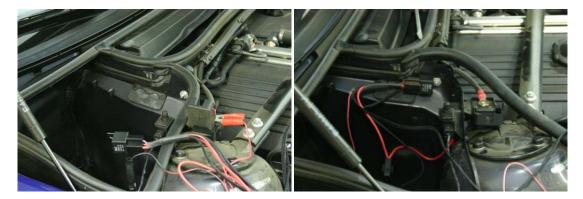
13. Mount the Angel Eye harness relay to the inner side of the empty compartment underneath the hood as indicated in the diagrams. The plastic shroud on the +12V terminal can be removed temporarily to attach the positive power lead with the black terminal ring going to chassis ground.
