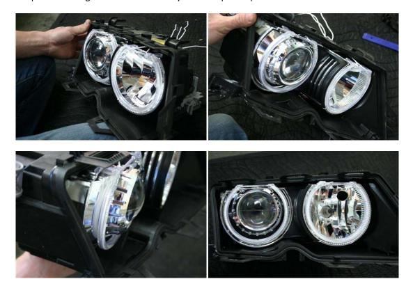
8. Here are completed images of the rings on the reflector housings. Aurora has a multi-stage clipping mechanism in order to align the clips perfectly onto your housings with interference from auto-leveling mechanisms.
