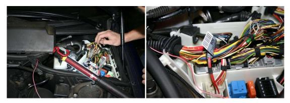
19. Remove the DME cover using a torx or allen bit (depending on model year) to expose the wiring. The red/white wire of the harness will be tapping into the red wire w/ white stripe - with yellow dots. Make sure the wire has the yellow dots before tapping.
