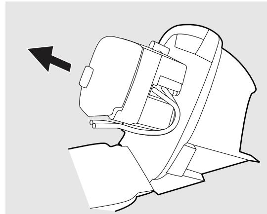
**7** Disconnect the two drainage tubes from the rear side of the blower assembly.
