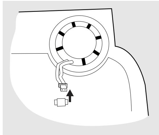
**5** Disconnect the two ribbon cables by loosening the connectors.
