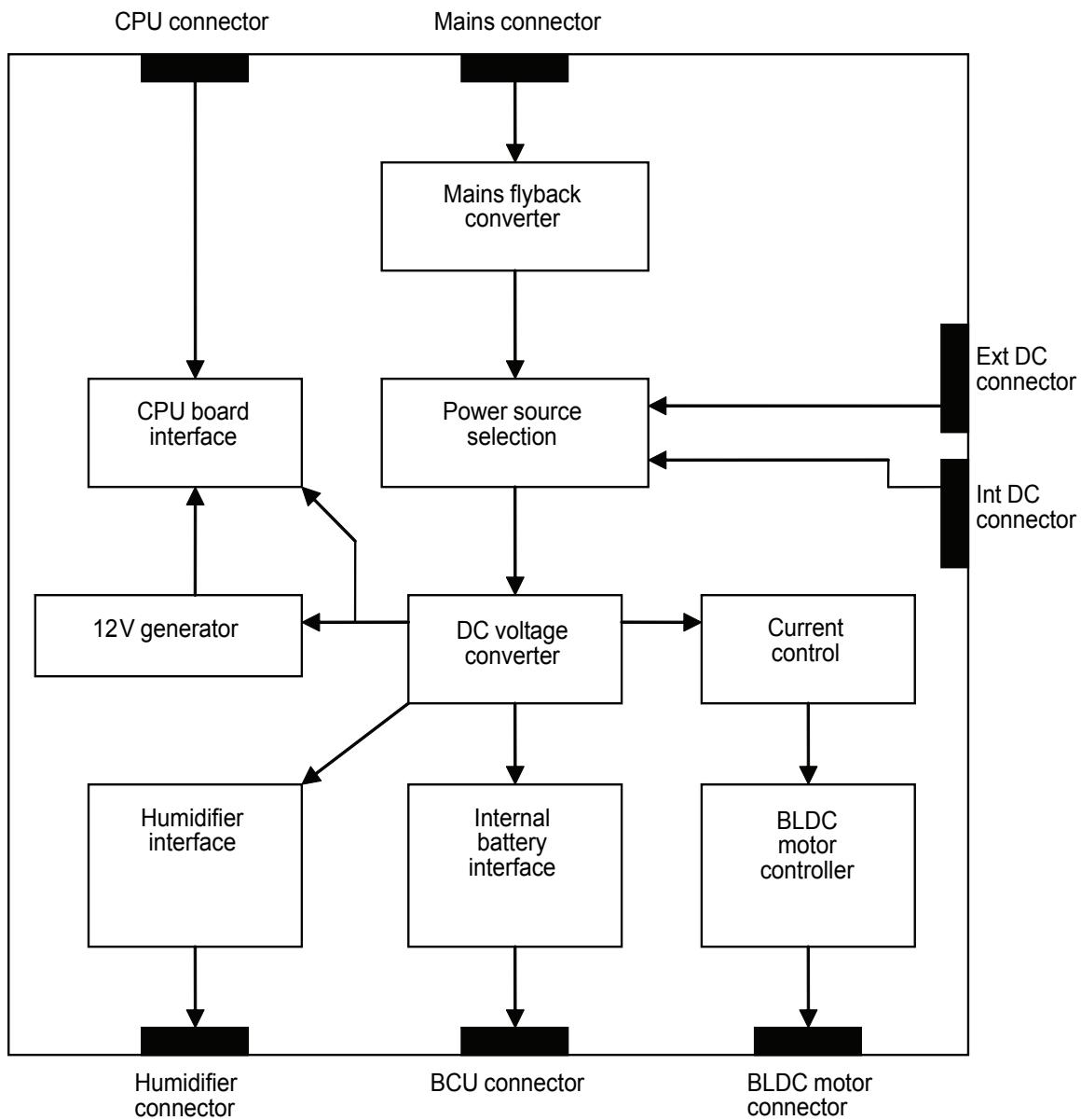
PSU board contains the switch mode power supply (SMPS) built on the double ended flyback topology. The converter is powered with mains 100-240 V AC, +10%, -20% (i.e. 80 V AC-264 V AC).
