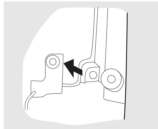
**5** Push the tube outlet through the hole at the rear of the Vivo 30/40.
