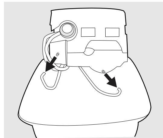
**8** Disconnect the BLDC motor control cable.
