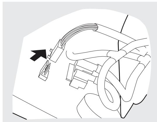
**3** Disconnect the yellow and the grey tubing at the T-connectors.
