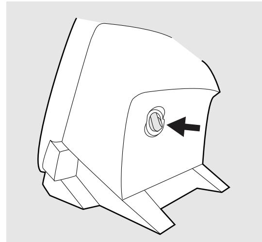
**6** Pull the complete blower assembly straight out.
