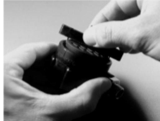
Figure 12 - Remove retaining ring
