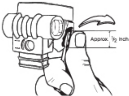
Figure 24 - Removal of exhaust cover - Step 1
