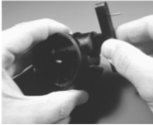
Figure 20 - Removal of cap plug
