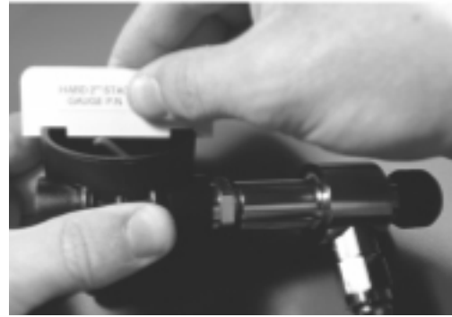
Figure 53 - Lever height setting (RH model)
