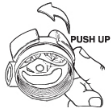
Figure 25 - Removal of exhaust cover - Step 2
