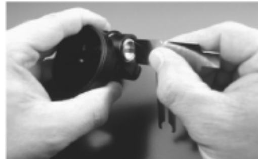
Figure 48 - Adjustment screw pre-set adjustment
