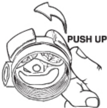
Figure 17 - Removal of exhaust cover - Step 2
