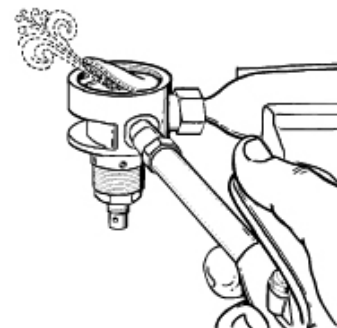
Figure 8 - Removal of diaphragm
