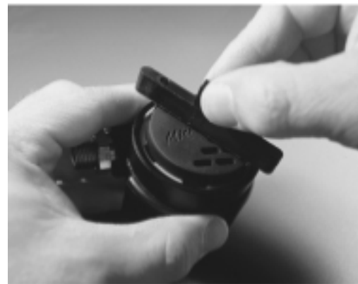
Figure 19 - Removal of retaining ring
