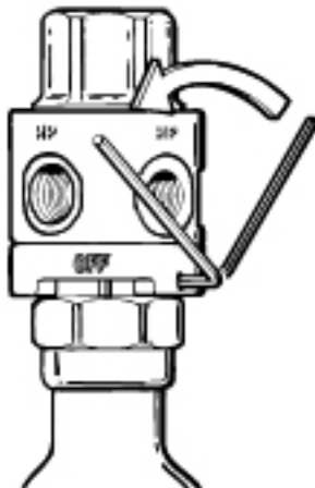
Figure 6 - Loosening indicator ring
