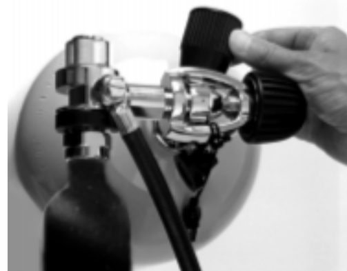
Figure 50 - SCUBA fill adapter connection with supply cylinder
