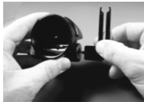
Figure 39 - Adjustment screw pre-set adjustment
