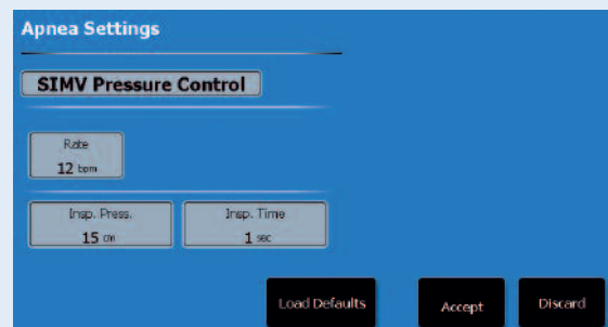
Adjustable apnea ventilation via inspiration time control
