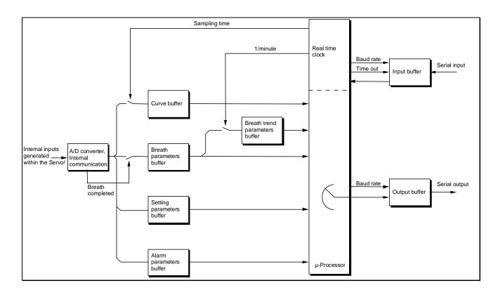
The information transfer between the CIE and the external equipment is performed via the serial communication link. The external equipment acts as the master and transmits commands to the CIE in order to retrieve information.
