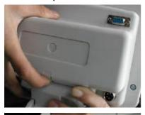
At first, release indicator from indicator bracket, like picture, then release 6 pcs screw from back cover of the indicator use cross
