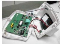
use iron solder off wire, bring new battery, use iron to solder the battery, (Attention: red line to positive electrode, black line to minus electrode), after check anything, plug the connector for power and try to turn on the power, if scale work correctly, replace battery completely.
