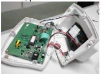
driver to put up the MPU from DIP40 socket (Attention: please don't let the IC pin tilt), then use the new MPU plug into DIP40 socket (Attention: please note the gap direction), after
