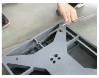
connector. Now, you can fix 8 pcs internal hexagon screw again (Attention: fix tight enough as you can ). Then you can check and adjust corner and overload stop use file and internal hexagon screw driver. After check anything, try to turn on the power and show the internal counts, if internal counts looks OK, close the pan, change load cell completely.
