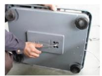
bracket, by this way, you can remove load cell now.
