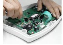
check anything is OK, plug the power connector (CH3.96 4P), try to turn on the power, if scale work correctly, replace MPU completely.
