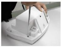
cover, pull of the connector for power (CH3.96 4P), use special IC kit or minus screw
