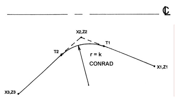
For the figure below, you program an Arc event from X1, Z1 to X2, Z2 with tool offset left, and another Arc event from X2, Z2 to X3, Z3 also with tool offset left. During the programming of the first Arc event, the system will prompt for Conrad at which time you input the numerical value of the tangentially connecting radius r=k3. The system will calculate the tangent points T1 and T2 and direct the tool cutter to move continuously from X1, Z1 through T1, r=k3, T2 to X3, Z3.
