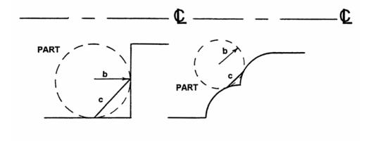
In both cases above a chamfer programmed with dimension b will cut a chamfer along line c.
