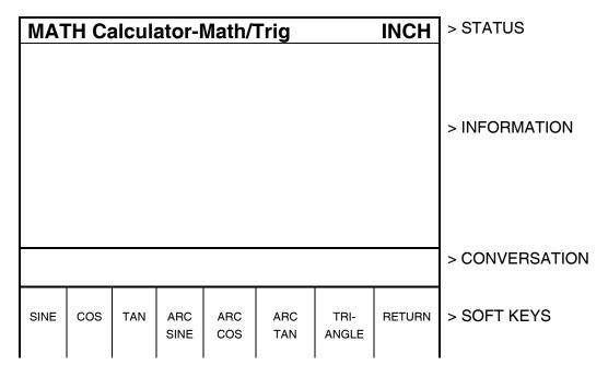
To calculate the sine, cosine or tangent of an angle, input the angle in degrees and press the **SINE**, **COS** or **TAN** soft key.
