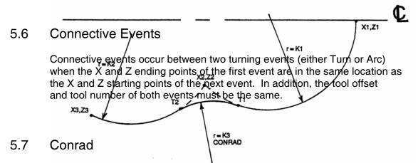
Conrad is a unique feature of the ProtoTRAK that allows you to program a tangentially connecting radius between connective events.
