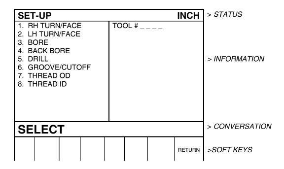
Input the tool type 1 through 8 and SET. If, for example, you chose 1 (the right-hand turn or face tool) the display would show:
