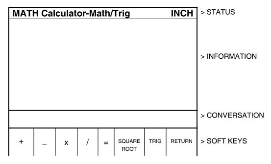
Use the soft keys like a simple calculator, but always press = for each calculation. Press **RSTR** to Clear Entry. For example, for
