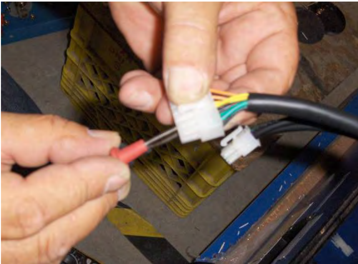
Fig. 3: For position 5 locate the green and black wires, with DVM on ohms position. Make sure switch opens and closes when it sees the notch.
