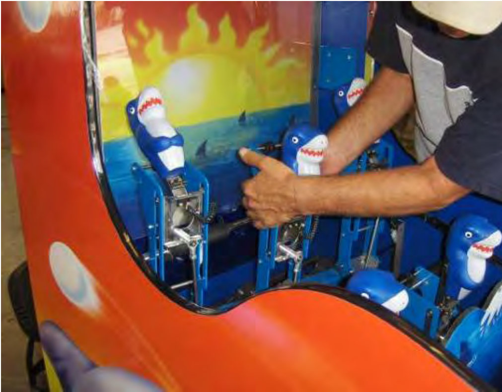
Fig. 10: Removal of shark head motor and sensor assembly from game
